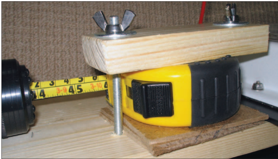
Fig. 2: The measuring tape's casing should be held in place via a pair of long screws terminated with wing nuts. This is so that the position of the tape can be fine tuned. The tape casing is finally clamped in place between the coupler and the base of the fishing rod, as shown in this diagram.
