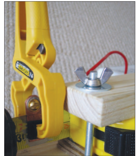
Fig. 3: The coating on the tape measure is removed at the area where the copper strips are clamped on to provide electrical contact (see text).
